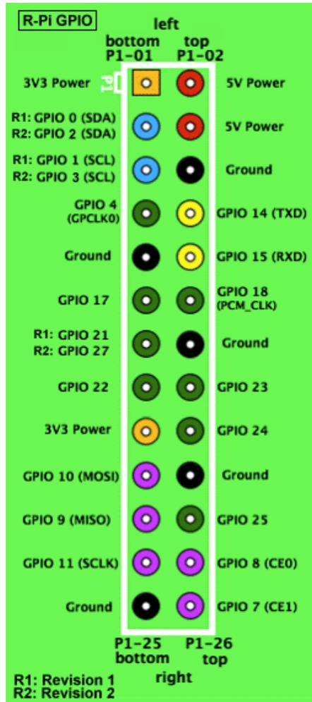
These pins are a physical interface between the Pi and the outside world. At the simplest level, you can think of them as switches that you can turn on or off (input) or that the Pi can turn on or off (output). Seventeen of the 26 pins are GPIO pins; the others are power or ground pins.
